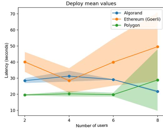
Fig. 3. Deploy mean latencies.
